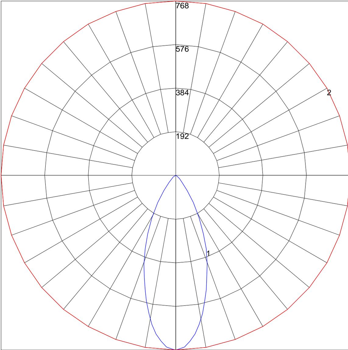
Maximum Candela = 768.16 Located At Horizontal Angle = 0, Vertical Angle = 0
