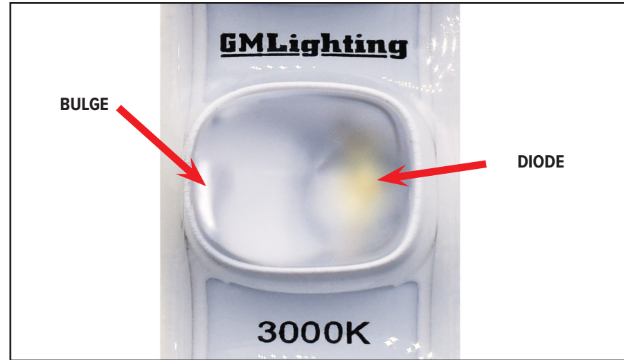
Note that yellow LED diode is opposite of the optic bulge.
